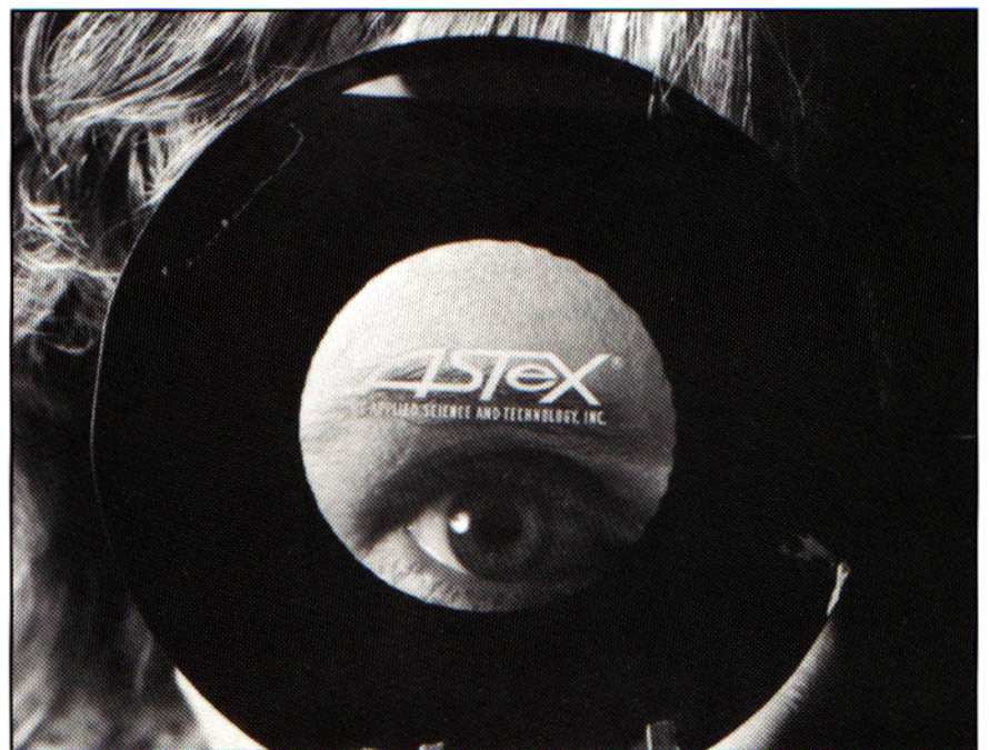
Diamond membrane approximately 2 µm thick. (Membrane courtesy of Dr. Henry Windischmann, BP America, Inc.)
